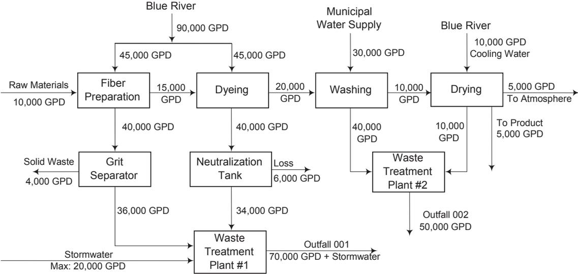
Schematic of Water Flow
