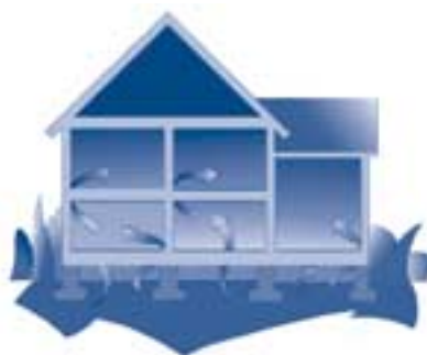
Figure 7. Radon Routes into a Home
